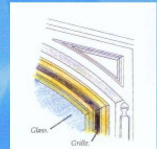
Detail of window frame with guide track
