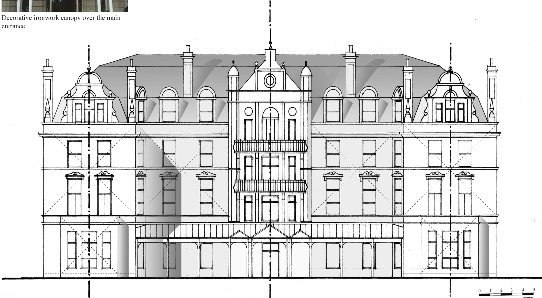
Typical 'tripartite' facade, composed of three main parts: two projecting wings and an entrance bay in high relief. A glazed canopy with decorative ironwork links the two wings.
