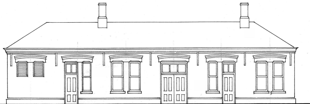
A typical GWR 'standard' station building (some components standard), brick built with stone dressings, hip roof and canopy.
