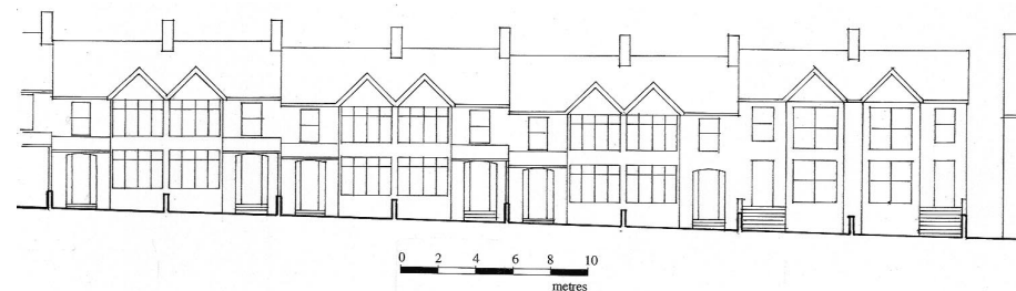
2-bay handed pairs (9C). The eaves line breaks with each pair of houses. Joined bay windows and doors to the outside of the pairs.
